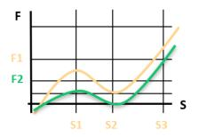
The patented function "IForce Calibration" is able to compensate the magnetic cogging forces, the load and the friction forces of the ROTAX® Rxhq direct drive in a very simple way. This makes it possible to limit and monitor torques in processes. Together with the XENAX® servo controller, complete torque/displacement diagrams can also be recorded an additional sensor is not necessary.
