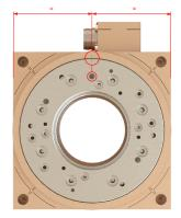
on. Therefore, no reference drive is necessary. For the alignment of the rotor flange, a single bore Ø4H6 with aligned marking on the shaft and a marking on the symmetry axis of the housing is provided. The absolute zero point is in straight alignment of the two markings.
