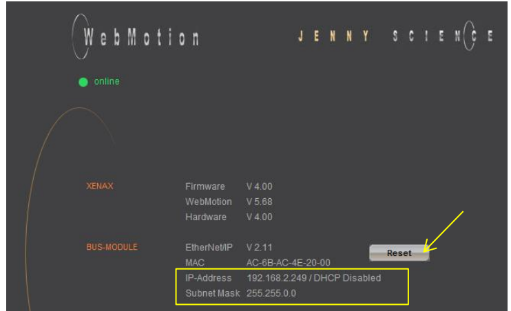
Communication parameters before reset (DHCP disabled, static IP Address 192.168.2.249)
